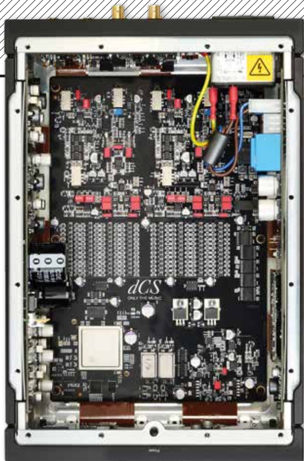
LEFT: The Lina network DAC employs a StreamUnlimited 800 series platform [right, sidewall]. More familiar, the 96 current sources (a 2x48 matrix) that comprise the RingDAC core [centre] are addressed via a Xilinx Artix-7 FPGA [lower left]. Note also the 48kHz/44.1kHz clocks [bottom]. Fully balanced, mixed op-amp analogue output [top] has its own regulated PSU
